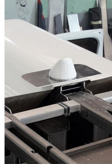
Figure 4 Dome Antenna (GPS, 3G/4G)
